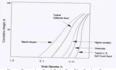
Fig. 14: Formation Sand Grain Size Distribution Curve
